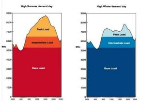
Figure 2: Load curve (courtesy of alfin2300.blogspot.com) [3]
